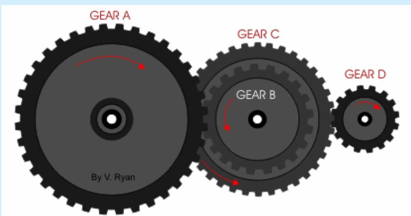
An example of a two-stage gearbox. Notice the difference in rotation speeds of the gears and their directions.
