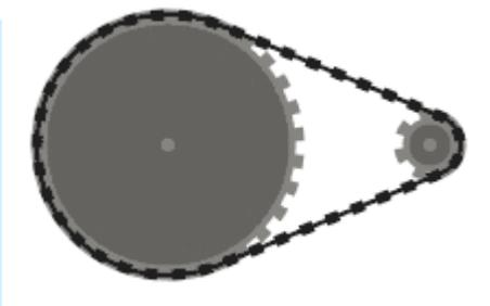
An example of a one-stage chain reduction, with the large sprocket rotating much slower than the small sprocket, but notice the chain moves the same speed all around.
